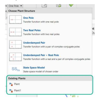
If the plant you select is a process model (idproc object), **PID Tuner** uses its structure. If the plant is any other model type, **PID Tuner** uses the state-space model structure.
