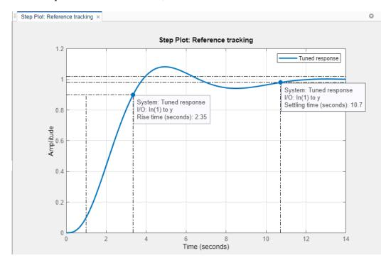
The initial PI controller design provides a rise time of 2.35 s and settling time of 10.7 s. Both results are slower than the design requirements.
