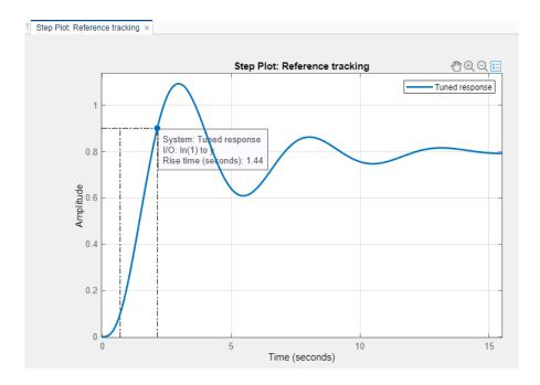
Moving the **Response time** slider far enough to meet the rise time requirement of less than 1.5 s results in more oscillation. Additionally, the parameters display shows that the new response has an unacceptably long settling time.
